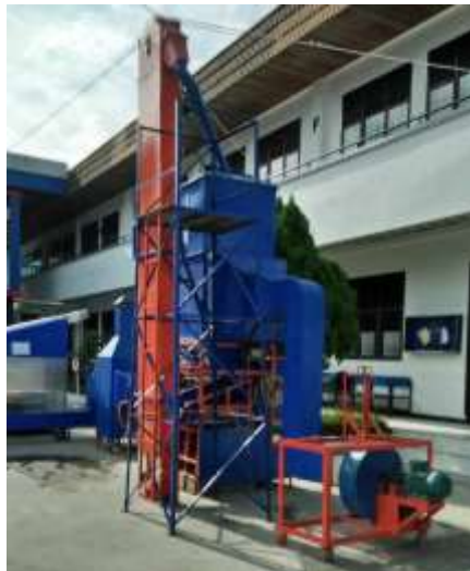
Fig. 1. Photograph of the solar hybrid recirculating mixed-flow dryer (SHRMFD).
