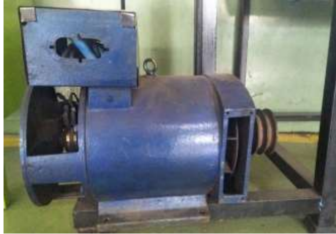
Fig. 1 - AC Generator 3kW 1-Phase
