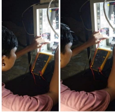
Fig. 11. Testing Sensor Output Voltage
