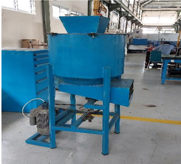
Fig. 5. Assembly results of the candlenut shell breaking machine
